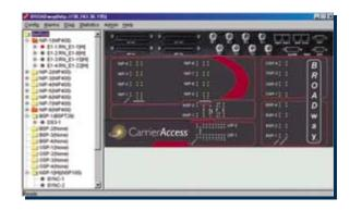
The Web-based GUI built into *BROAD* way provides the most convenient and intuitive way to manage the system. All management functions are available from this interface and users can configure new circuits, check alarms, run diagnostics, and set up protection schemes. The GUI also allows a remote technician to view front panel indicator LEDs in real time. In addition, an online, context sensitive help system is in place to guide the user through all aspects of the system.
